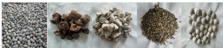
Figure 1. Wetland fillers, in order of ceramic, volcanic rock, lapis lazuli, sulfurous iron ore, and polyaluminum chloride composite filler.
