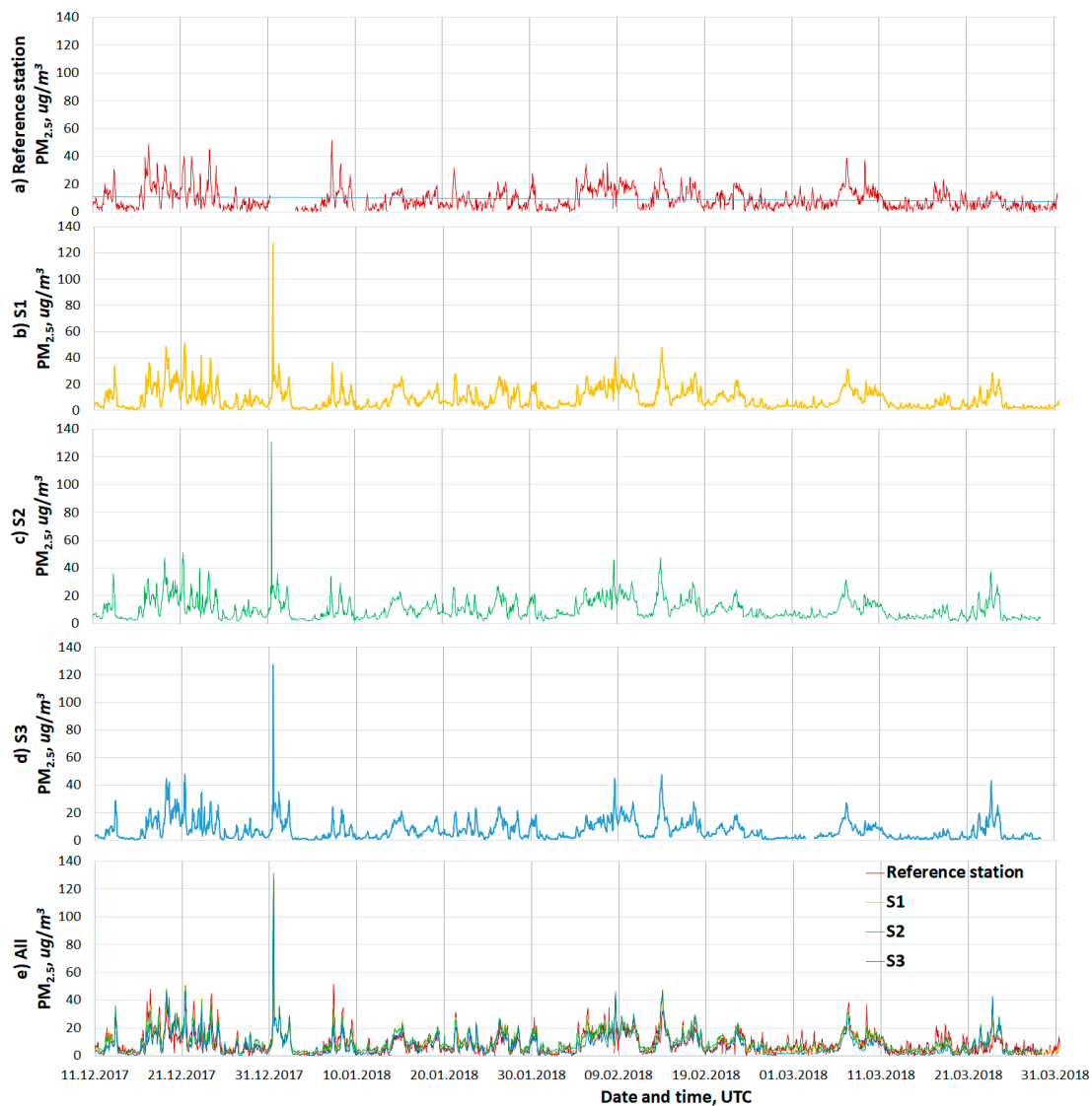
Figure 4. Results of PM_{2.5} measurement from three SDS011 sensors and an official reference monitoring station in the period of 11 December 2017 to 31 March 2018: (a) Official reference station; (b) S1; (c) S2; (d) S3; (e) Comparison among the official reference station and three SDS011 sensors. 1 h averaged data was plotted.
