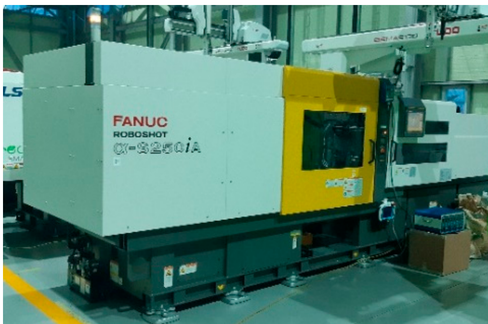
Figure 4. A photograph of injection molding machine used (ROBOSHOT α-S250iA, FANUC).
