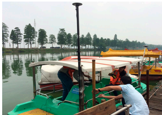
Figure 15. The test environment of shipboard kinematic PPP.
