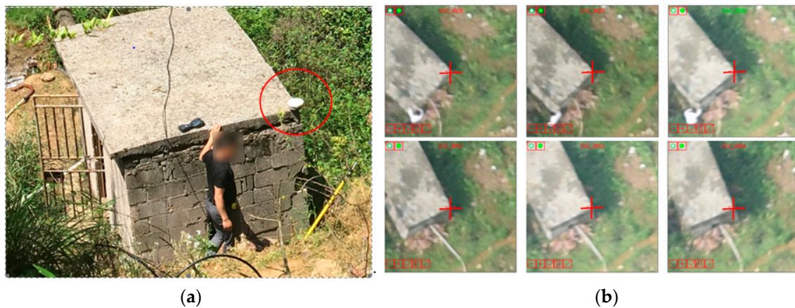
Figure 14. The location and image measurement of GCP No. 9012. (a) The location of No. 9012; (b) The image measurement of No. 9012; the red crosses represent the location of the GCP in the images.
