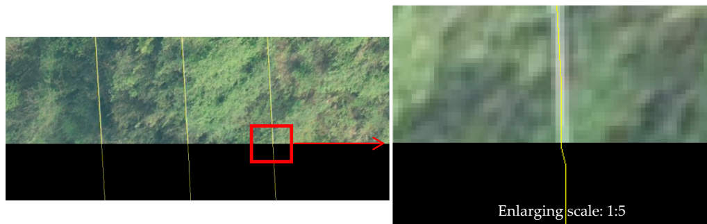
Figure 15. Registration of a 2D vector and epipolar images of the power line.
