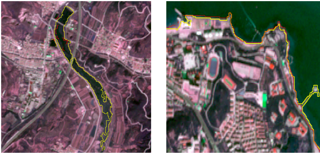
Figure 13. The comparative boundary extraction results of the proposed NDWII method and traditional NDWI method from the Sentinel-2 image (true color synthesis) of Yantai. The yellow lines present the result using the proposed NDWII method, whereas the red lines show the results using traditional NDWI (10 m).
