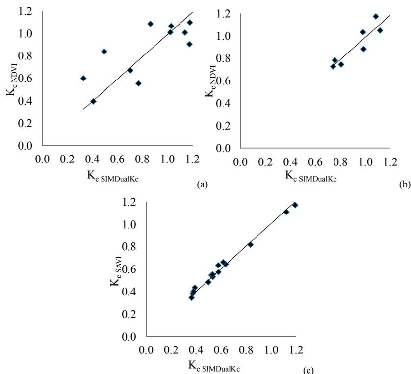
**Figure 7.** Comparison of actual  $K_c$  derived from SIMDualKc ( $K_{c \text{ SIMDualKc}}$ ) and actual  $K_c$  derived from the combined approach of  $K_{cb \text{ VI}}$  and  $K_e$  from SIMDualKc ( $K_{c \text{ VI}}$ ) for (a) maize; (b) barley; and (c) olive.
