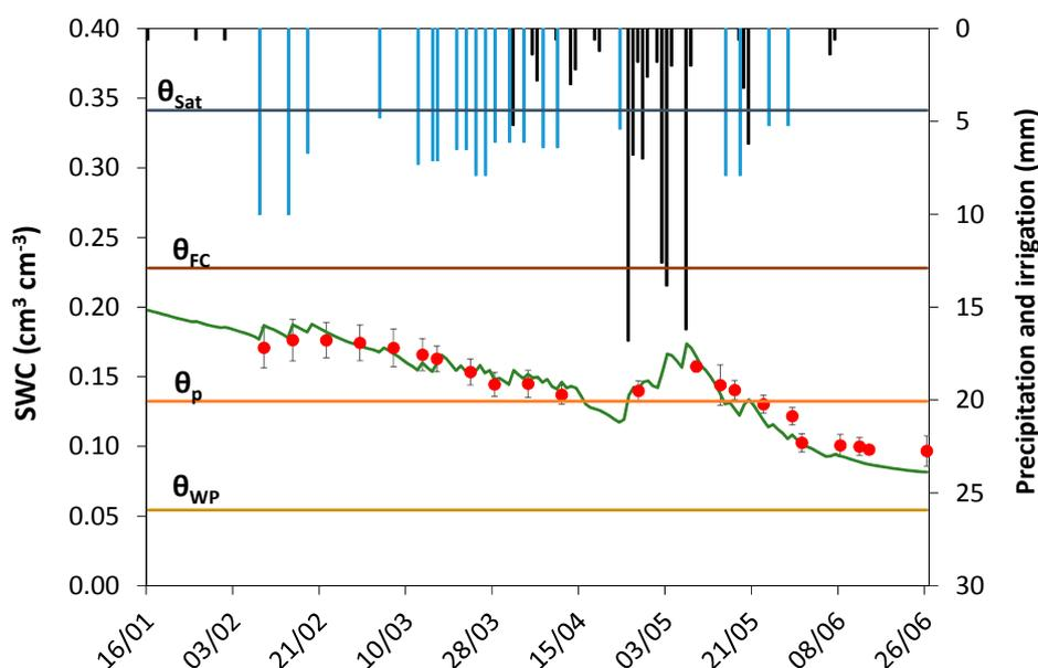
**Figure 2.** Observed (•) and simulated (—) daily soil water content (SWC) after the calibration of SIMDualKc for barley in the dry year (error bars correspond to the standard deviation of SWC observations);  $\theta_{Sat}$ ,  $\theta_{FC}$ ,  $\theta_p$  and  $\theta_{WP}$  are respectively the SWC at saturation, field capacity, wilting point and at non-stressed depletion fraction  $p$ ). Precipitation is represented by dark bars and irrigation by the light ones (source: [35]).
