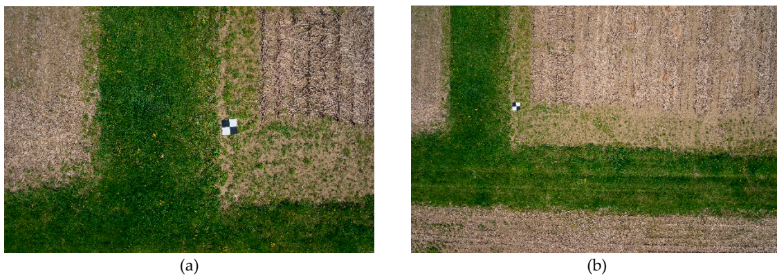
Figure 14. Sample images captured by the Sony RGB sensor over the calibration test field. (a) 20 m flying height and (b) 40 m flying height.
