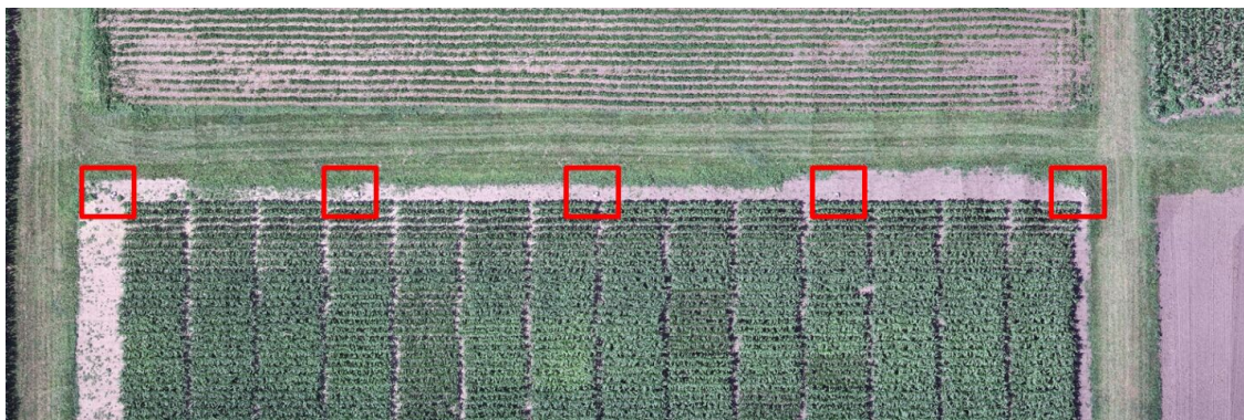
Figure 23. Orthophoto result from direct approach for FLIR RGB July 25th data collection (red boxes show the location of the check points, Original Image GSD \approx 0.01m ).
