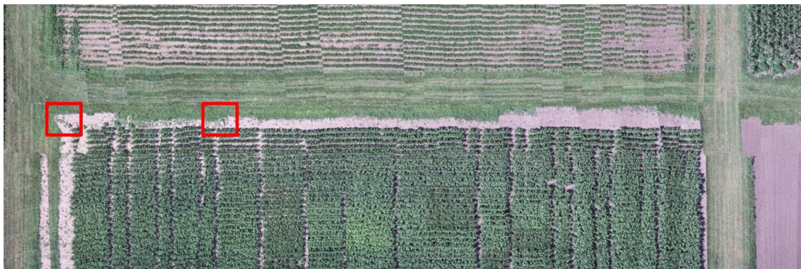
Figure 21. Orthophoto result ignoring the time delay using the original trajectory data for FLIR RGB July 25th data collection (red boxes show the location of the check points—only two visible, Original Image GSD \approx 0.01m).
