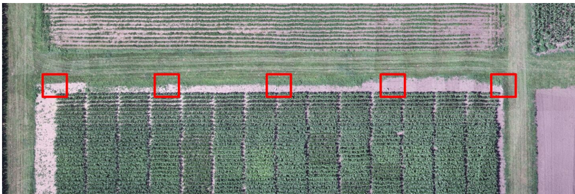
Figure 22. Orthophoto result ignoring the time delay using the refined trajectory data for FLIR RGB July 25th data collection (red boxes show the location of the check points, Original Image GSD \approx 0.01m ).
