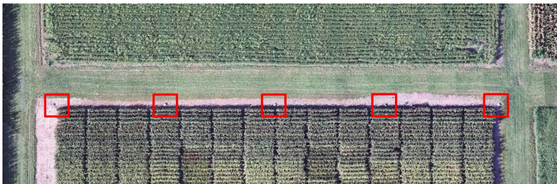
Figure 24. Orthophoto result from Direct Approach for FLIR RGB September 14th data collection (red boxes show the location of the check points, Original GSD \approx 0.01m ).
