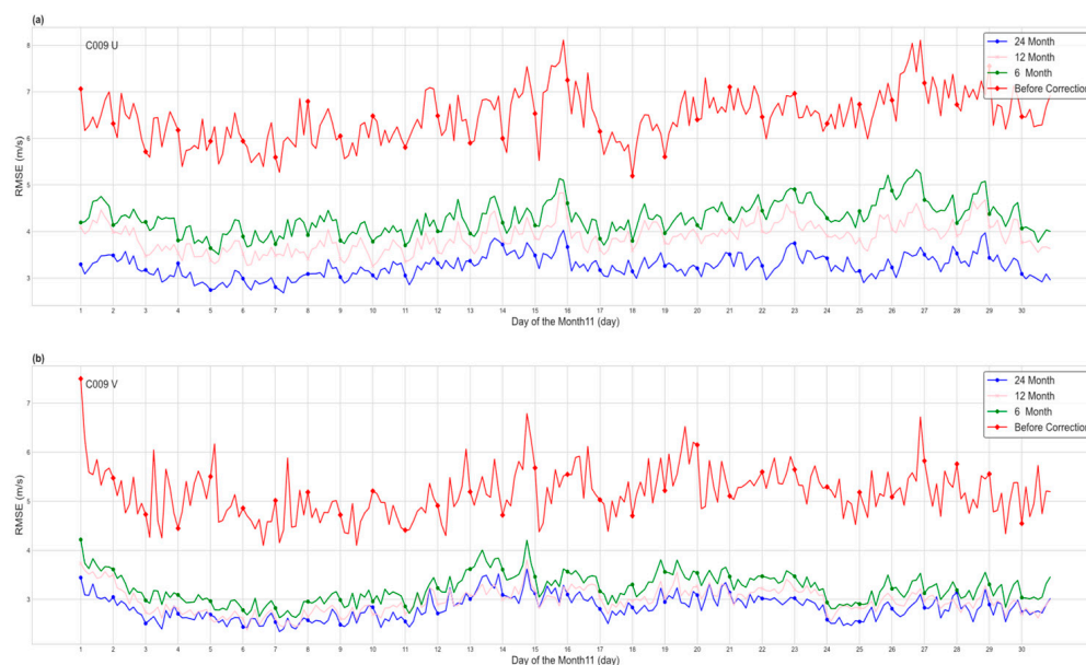
Figure 17. Analysis of model correction results with training data of different periods (red represents the original root mean square error, green represents the root mean square error corrected by the model trained with 6 months of data, pink represents the root mean square error corrected by the model trained with 12 months of data, and blue represents the root mean square error corrected by the model trained with 24 months of data).
