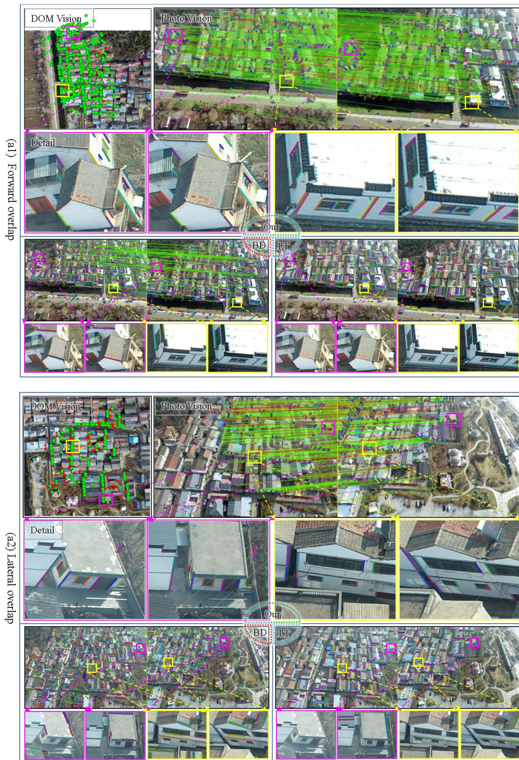
Figure 16. Matching results of township scene a. In the DOM vision, the green circles and red crosses correspond to the SPPs (which are also the projection results of the spatial plumb lines generated by the forward intersection of the homologous plumb-line pairs) corresponding to the correct and erroneous plumb-line pair matching results, respectively. In the Photo and Detail visions, the homologous plumb-line pairs are shown in the same color. In the Photo vision, the green and red connecting lines correspond to the correct and erroneous matching results, respectively. Figures 17 and 18 are similarly represented as such.
