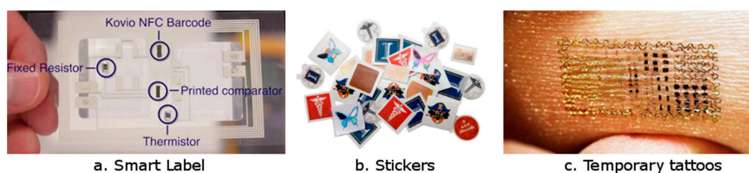
Figure 5. Comparison of micro-thin sensors. (a) Smart Label composition (b) Sensors embedded in stickers; (c) Sensor directly printed on the skin [76,78,84].
