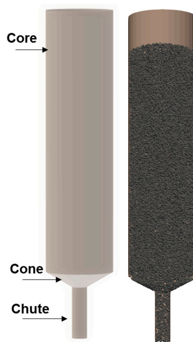
Figure 8. The CAD model of Xe-100 reactor walls ( left ) and the reactor loaded with over 200 hundred thousand fuel pebbles via DEM simulation ( right ).
