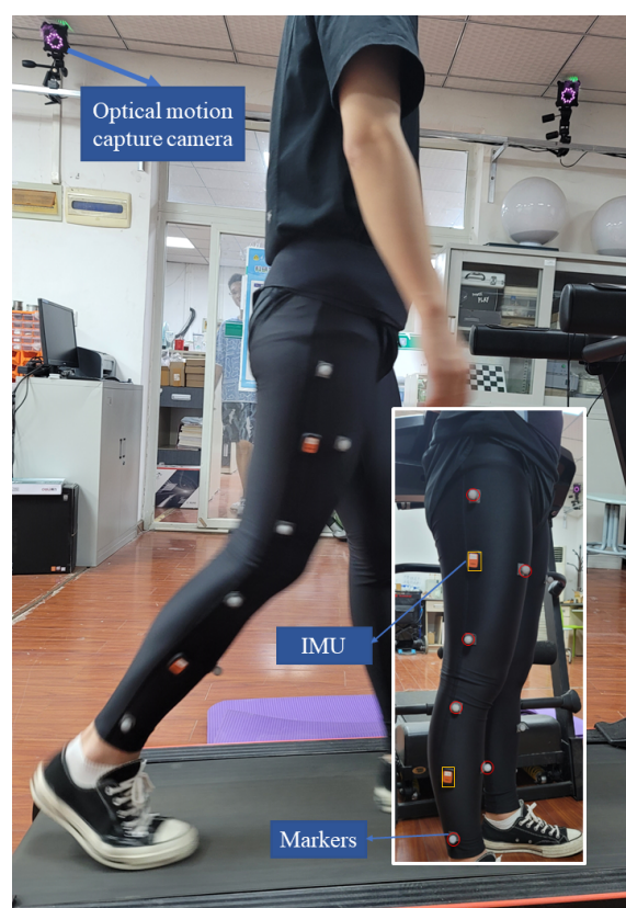
Figure 3. The experimental scenario mainly includes an optical motion capture system, IMUs and a treadmill; six markers and two IMUs are set on each leg, three markers on each segment are not co-planar and the direction of IMUs is not required.
