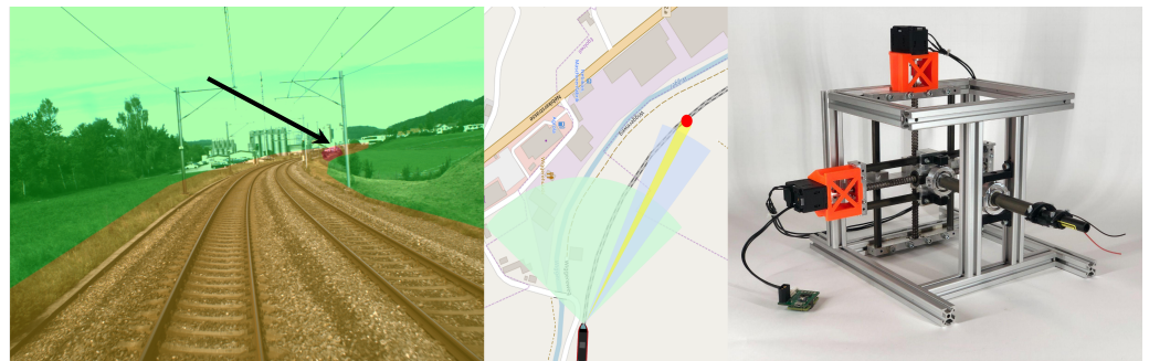
Figure 2. Long-Range Obstacle Detection systems need to focus their sensors on targeted Regions of Interest, shown in yellow and red (arrow), in the vicinity of the railway track. The change of attitude of individual sensors is shown in the centre image, to focus the sensors on possible obstacles. This can be done using a high precision pointing mechanism as shown on the right.
