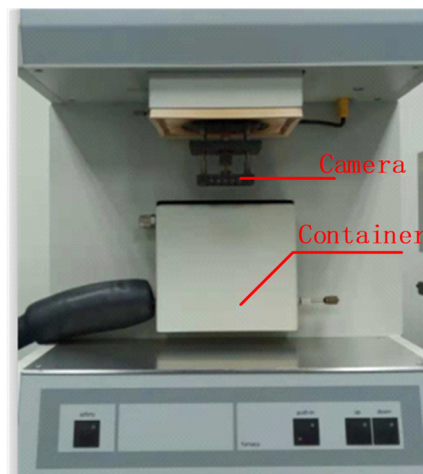
Figure 2. The equipment of creep experiment mainly consists of two parts, a high-resolution camera and a container. Camera can record the micro deformation of object in the container, and the container is a temperature-controlled oven which can provide precise temperature from -70 °C to +100 °C.
