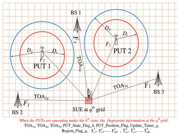
Figure 3. Grid-based sensing scenario and data collection.
