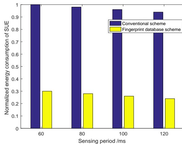
**Figure 8.** Power consumption of conventional sensing scheme and the wireless fingerprint database (WFPD) aided scheme with different sensing period  $T_s$ .
