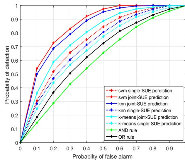
Figure 10. Receiver operating characteristics (ROC) of different sensing algorithms.
