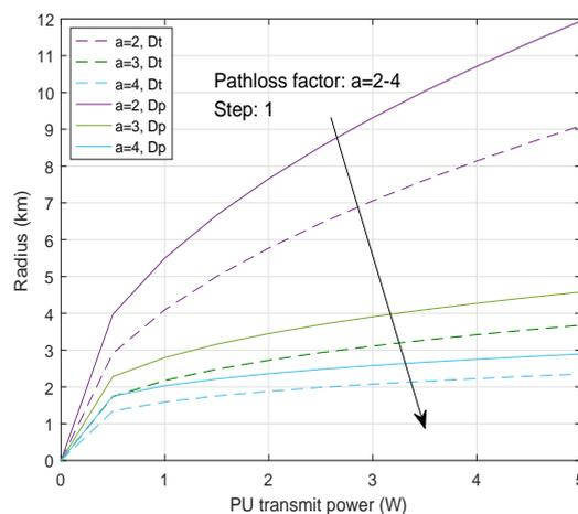
Figure 2. Relationship between the region radius and primary user transmitter (PUT) power.
