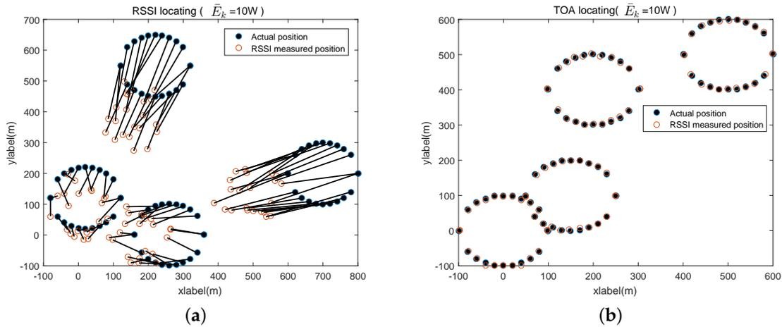
**Figure 7.** Accuracy comparison of TOA and RSS-based SUE positioning. (a) Accuracy of received signal strength (RSS)-based secondary user equipment (SUE) positioning. (b) Accuracy of time of arrival (TOA)-based SUE positioning.
