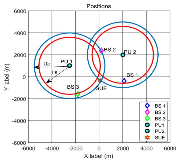
**Figure 5.** Spectrum sensing scenario in the cellular cognitive radio network (CCRN).
