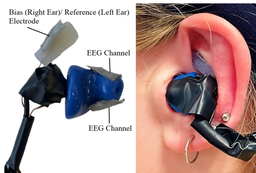
Figure 2. The earpiece design with a close-up of the earpiece on the (left) and how it fits in the ear on the (right).
