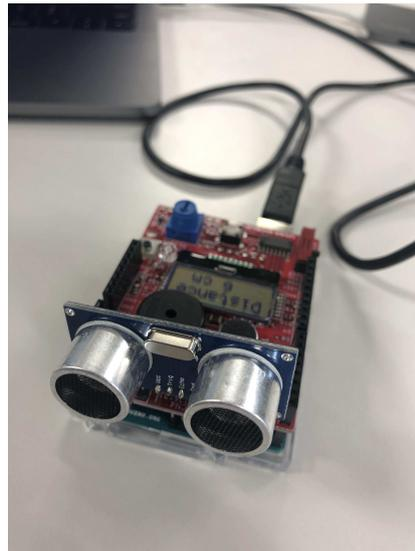
**Figure 7.** A distance measuring sensor.
