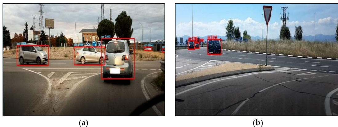
Figure 8. Snapshots of vehicle detection using the You Only Look Once (YOLO) framework, (a) Vehicles in front of and to the right, (b) Vehicles to the right.
