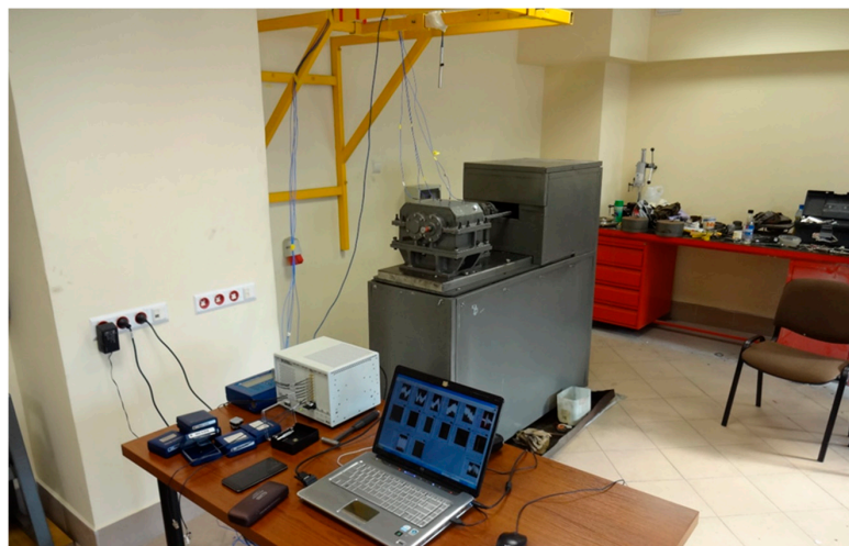
Figure 1. View of the FZG stand and the measuring system for stand tests [59].
