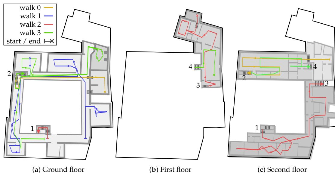
Figure 8. All conducted walks within the building. The arrows indicate the running direction and a cross marks the end. For a better overview we have divided the building into three floors, which are connected by four stairs (numbered 1–4). However, each floor consists of different high levels. They are separated from each other by different shades of grey, dark is lower than light.
