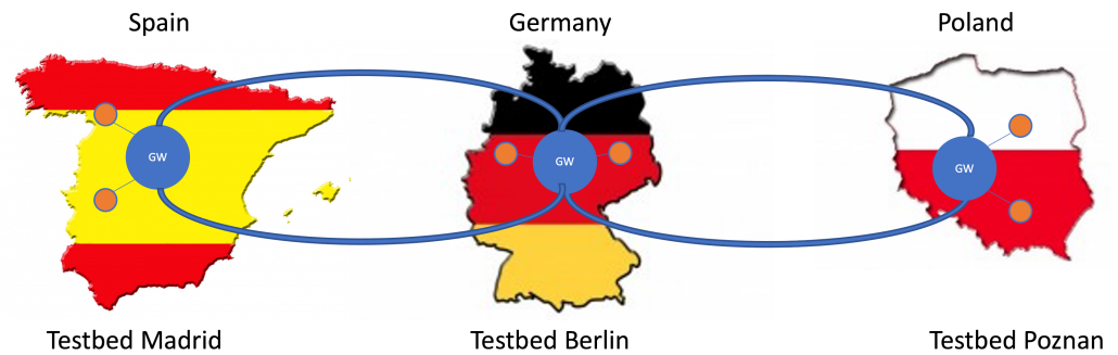
Figure 1. Connection of the quantum testbeds in Madrid (left), Berlin (middle), and Poznan (right) with emulated long-distance QKD links. The key exchange is indicated by the curved blue lines, which connect dedicated QKD gateway nodes (blue circles) in each testbed. The other QKD nodes in the respective testbeds are indicated by orange circles.
