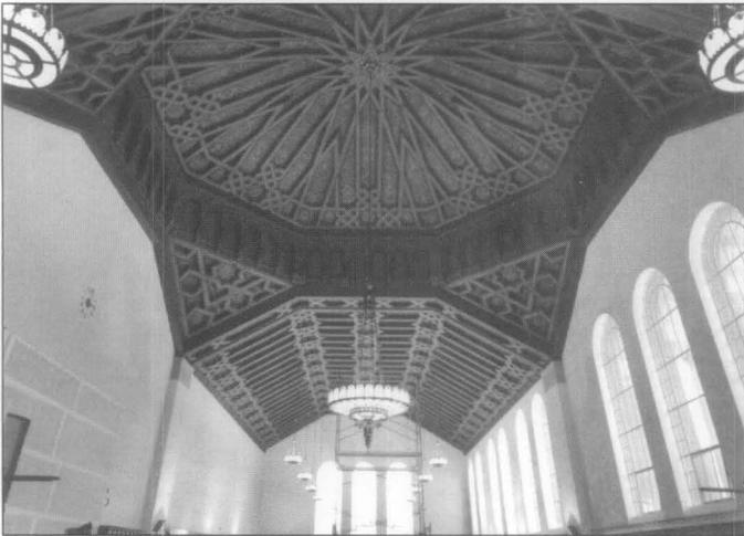
16. During the extensive rehabilitation of this historic building, new concrete, behind the new plaster finishes, strengthened the exterior brick walls and additional roof reinforcement was hidden behind the repaired/reconstructed coffered ceiling. Photo: © Jonathan Ferrar, courtesy UCLA Capital Programs.
