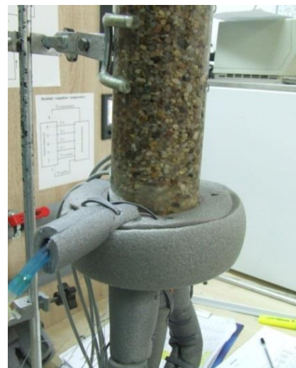
Figure 9. A porous granular bed filling the test chamber
