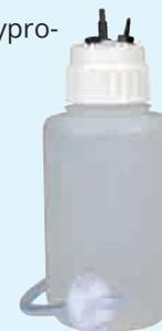
2l borosilicate glass collection bottle with high chemical resistance, with splinter-proof coating, special bottle head for minimized foam and aerosol formation, hose nozzle for VacuuHandControl VHC<sup>pro</sup> and additional port to connect a second VHC<sup>pro</sup> (optional), hydrophobic filter element 0.2 µm to protect pump and environment, hose for connection to pump unit BVC or BVC basic; fully autoclavable.
