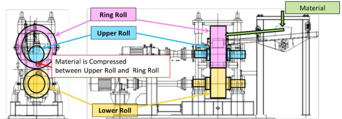
Figure 4 Component of Nippon Steel & Sumikin Engineering Squeezer
