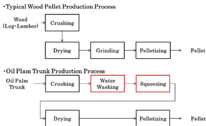
Figure 1 Comparison of Pellet Production Process
