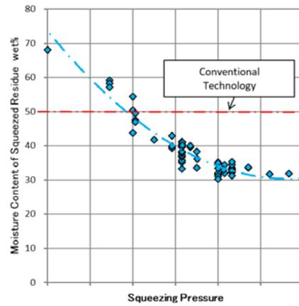
Figure 7 Relation between Squeezing Pressure and Moisture Content of Squeezed Residue
