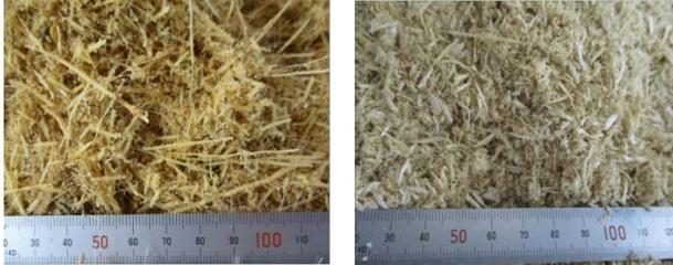
Figure 9 Crushed Chip and Squeezed Residue (Photo)
