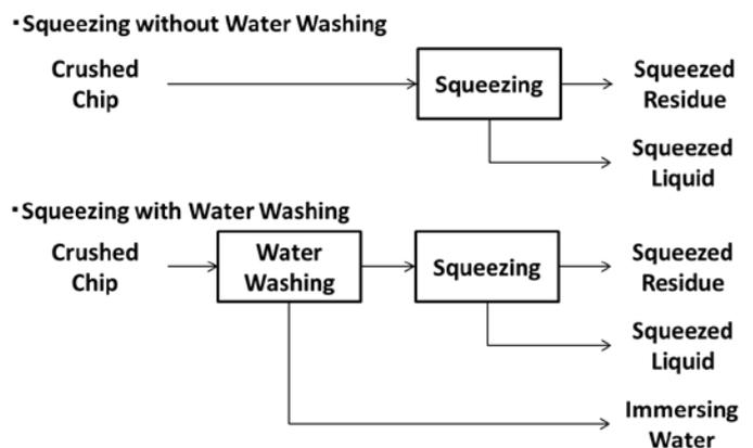
Figure 12 Potassium Reduction Test Flow
