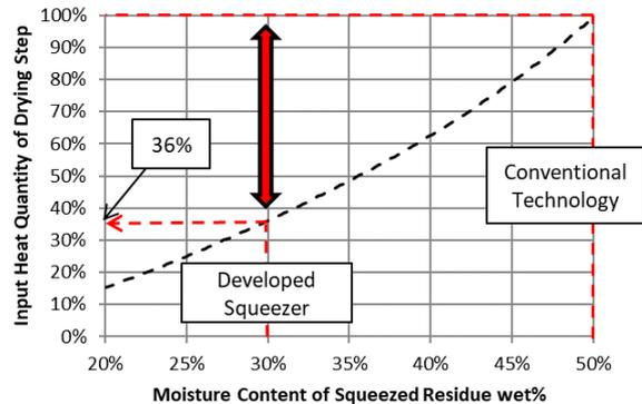
Figure 8 Required Heat Quantity Comparison between Nippon Steel & Sumikin Engineering Squeezer and Conventional Technology
