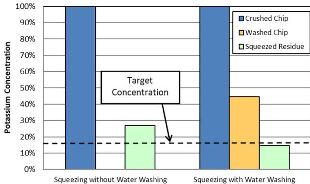
Figure 13 Potassium Reduction Test Result
