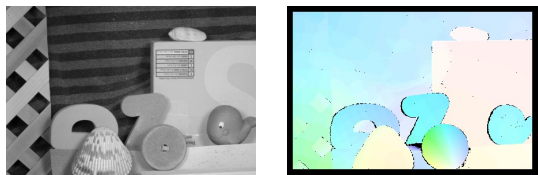
Figure 3. Seashell : A second example of a sequence captured using hidden fluorescent texture. We display the first frame (left) and the color-coded (see Figure 1) ground-truth flow (right).
