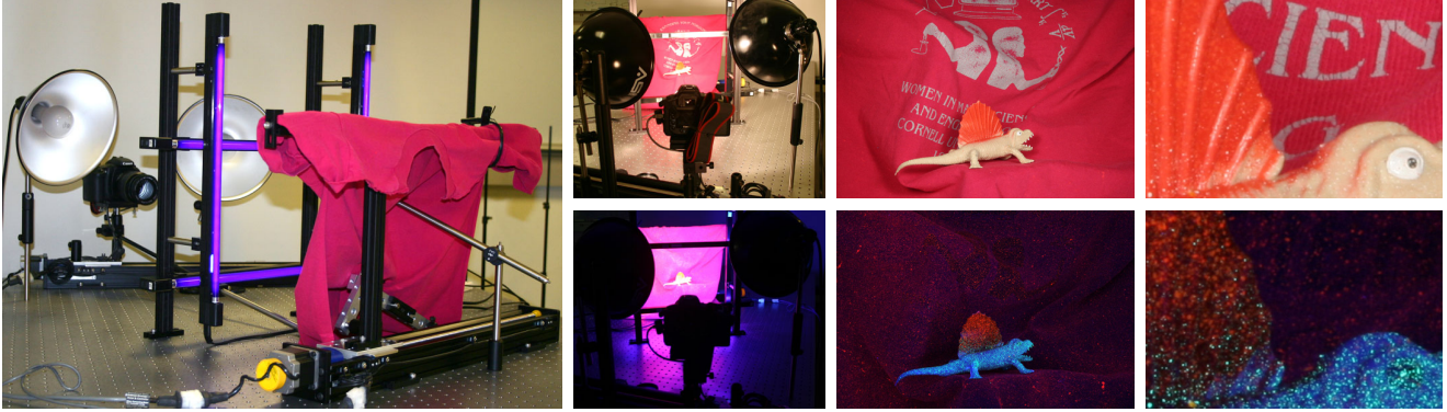
Figure 2. Our setup for obtaining ground-truth flow using hidden fluorescent texture, including computer-controlled lighting and motion stages for camera and scene. The small images show visible light illumination (top row) and UV illumination (bottom row); the middle column shows the high-resolution images taken by the camera, and the right column shows a zoomed portion. The high-frequency fluorescent texture in the UV images allows accurate tracking, but is largely invisible in the low-resolution test images.
