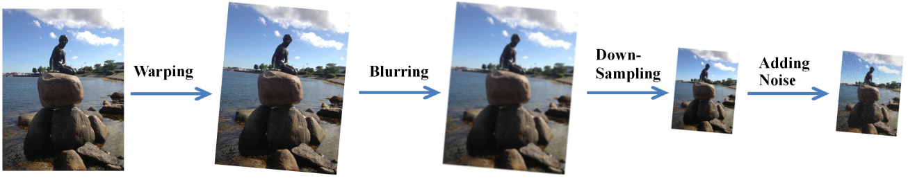
Fig. 3 The imaging model employed in most SR algorithms.
