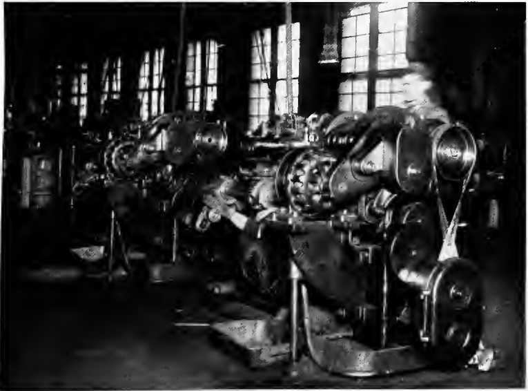
TURRET LATHES, ALL GEARS GUARDED
