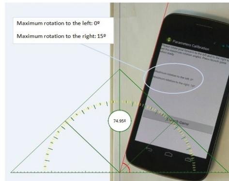
Figure 5: Photo of validation of a rotation measured by the smartphone.
