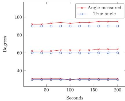
**Figure 6: Comparison between angles obtained from sensor fusion and real angles.**
