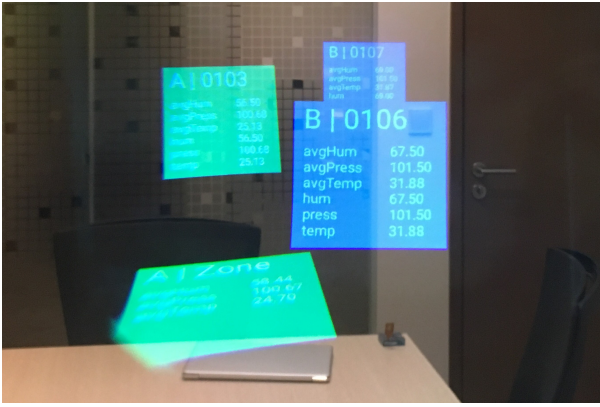
Fig. 6: Interface of the augmented reality dashboard
