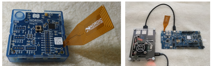
Fig. 3: (a) Thingy:52 as a mesh node, (b) Raspberry Pi with nRF52840 DK as the gateway
