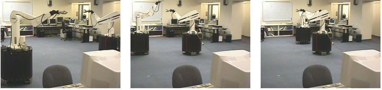
Figure 3: Obstacle avoidance behavior using the elastic strip framework is demonstrated on the Stanford Robotic Platform. The experiment corresponds to the one shown in Figure 2.
