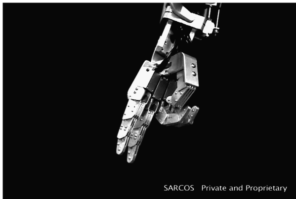
Figure 3. Five-finger humanoid robot hand with 6 d.o.f. (built by SARCOS).
