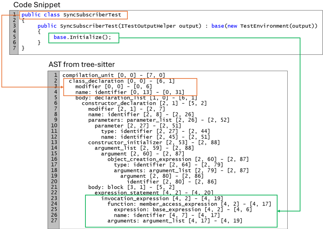
Fig. 5. AST structure for a C# code snippet produced by tree-sitter.
