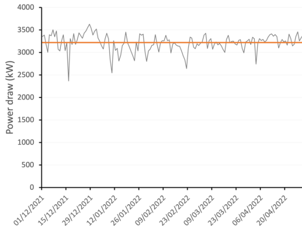
Figure 1: Measured power draw of ARCHER2 compute cabinets for Dec 2021 – Apr 2022. Orange line indicates mean power draw (3,220 kW).
