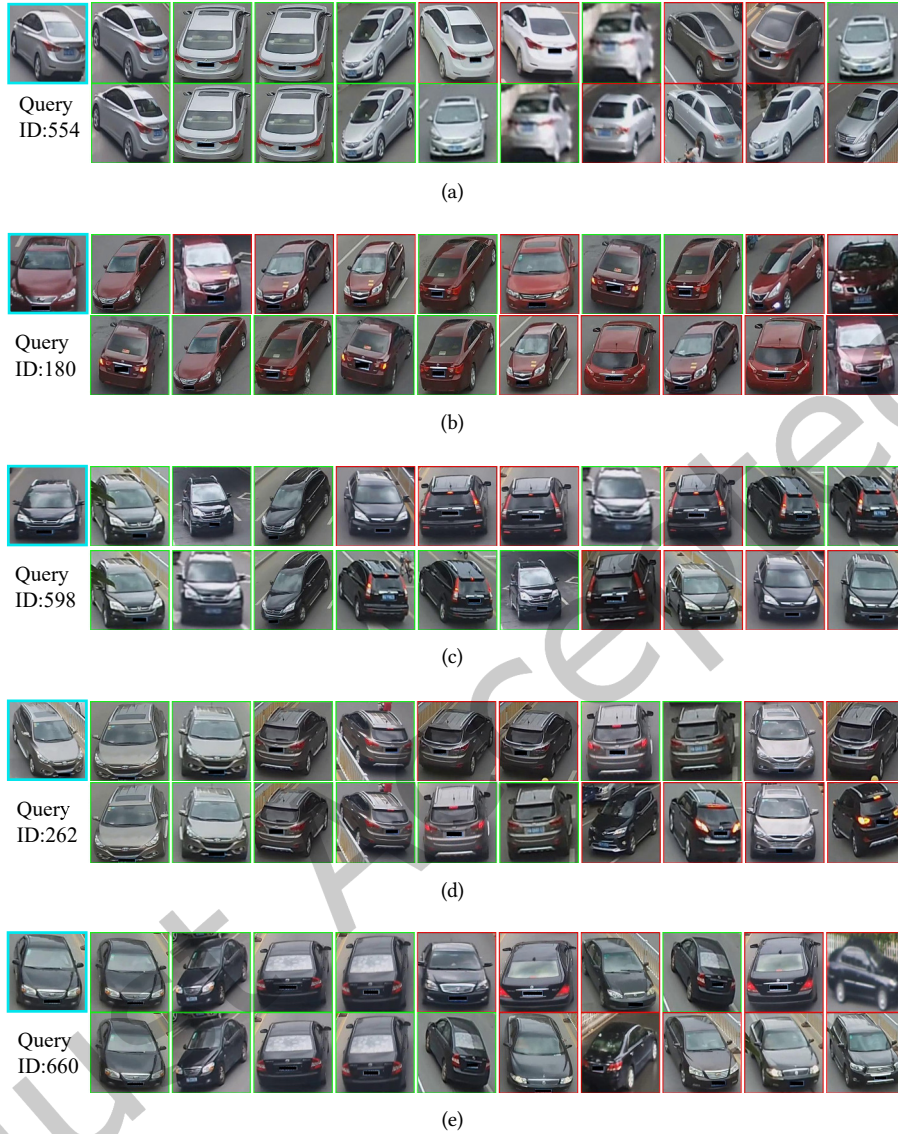
Fig. 6. Examples of Rank-10 retrieval results on VeRi-776 in multi-gallery-shot representations. The top row in each example of queried vehicle image represents the results of the baseline while the bottom row illustrates the retrieved vehicle images by the proposed SSR-Net model.
