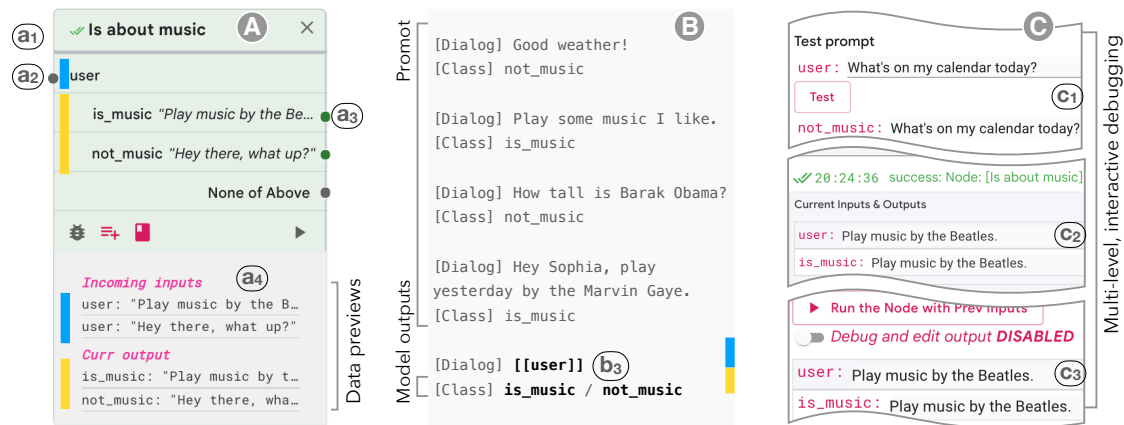
Figure 4: An expansion of Figure 2, is about music: (A) Node visualization: the node has a status icon ( a_1 ), a list of named input ( a_2 ) and output handles ( a_3 ), as well as detailed data previews ( a_4 ). (B) Implementation: the handle names are synchronized with the underlying prompt template ( b_1 ). (C) We can debug the node at multiple levels.
