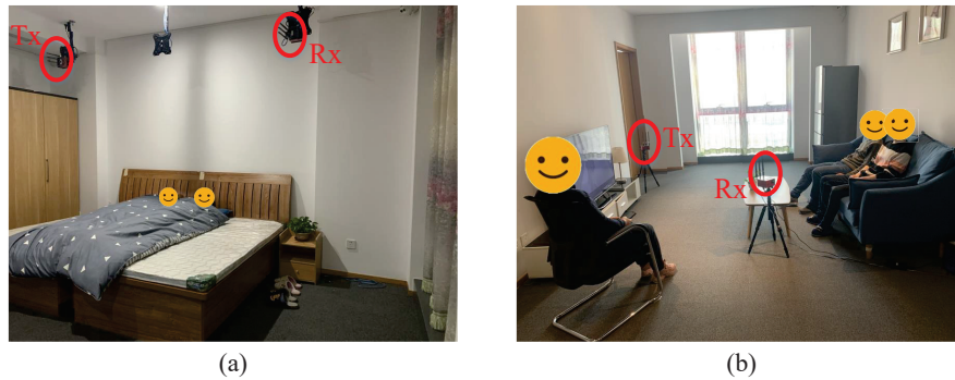
Fig. 14. The experimental setup in two scenarios: (a) all subjects sleep on a bed in the bedroom; (b) each subject sits on a couch or chair in the living room.
