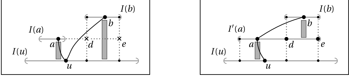
Figure 17: A step in the general transformation and the maintenance of invariants. (left) Before the transformation: a and b are children of u in T . Crosses mark locations of newly added points d and e . (right) After the transformation: b is a child of a in T' . Intervals shown as horizontal segments, respecting tree-structure (Invariant (1)). Shaded rectangles indicate empty areas (Invariant (3)). Smaller dots indicate interval endpoints and their projections (Invariant (4)), some points omitted for clarity. Non-emptiness of newly created rectangles (Invariant (2)) is guaranteed by newly added points and the points of Invariant (4).
