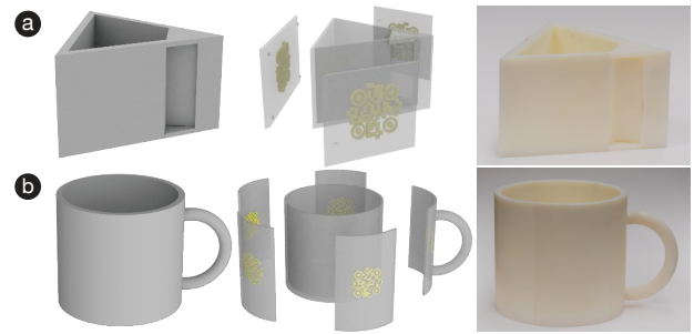
Figure 3. Multiple AirCode tags are embedded in a triangular drawer (top) and a mug (bottom). These tags are unique from each other. As long as one of the tags can be viewed by the camera system from a view angle, the object can be recognized and its pose can be estimated.
