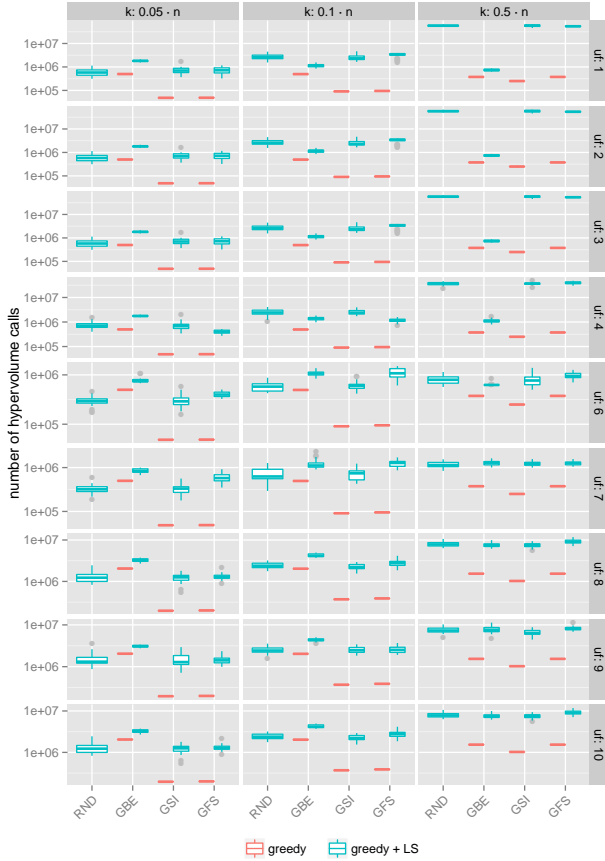
Figure 5: Number of hypervolume calls (in log-scale) performed by each heuristic for structured instances.
