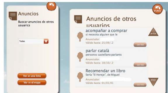
Figure 2. The Life2.0 interface with a list of help offers and requests created by the participants. By clicking on one of them, the user can write a comment or send a direct message to the author of the announcement.
