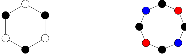
Fig. 2: The 6-cycle of alternating damped (black) and undamped (white) nodes is PI-GAS. On the other hand, the similar 8-cycle allows oscillatory behavior, as can be shown with the above richly balanced colored graph.
