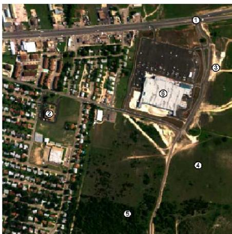
Figure 5: Urban data set taken from an aircraft (army geospatial center) with road surfaces (1), roofs 1 (2), dirt (3), grass (4), trees (5) and roofs 2 (6).
