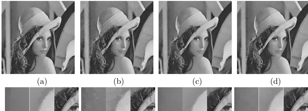
FIG. 4.6. Reconstructions using different choices for \kappa_{\mathcal{F}} in Step 1 of the proposed approach for the noisy image in figure 1.4. (a) \kappa_{ROF} = \kappa(\text{ROF}(I)) , PSNR=29.39 , PIQ=69 . (b) \kappa_{ROF} = \text{ROF}(\kappa(I)) (proposed approach), PSNR=29.41 , PIQ=92 . (c) \kappa_{NLM} = \kappa(\text{NLM}(I)) , PSNR=30.32 , PIQ=80 . (d) \kappa_{NLM} = \text{NLM}(\kappa(I)) (proposed approach), PSNR=30.86 , PIQ=103 .
