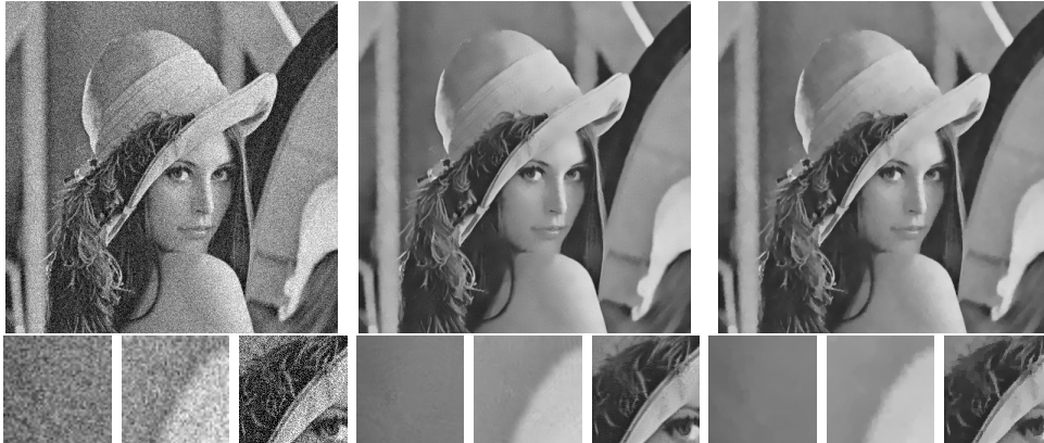
FIG. 4.3. Left: noisy image. Middle: result obtained with NLM denoising of the image. Right: result obtained with NLM denoising of the curvature image.
