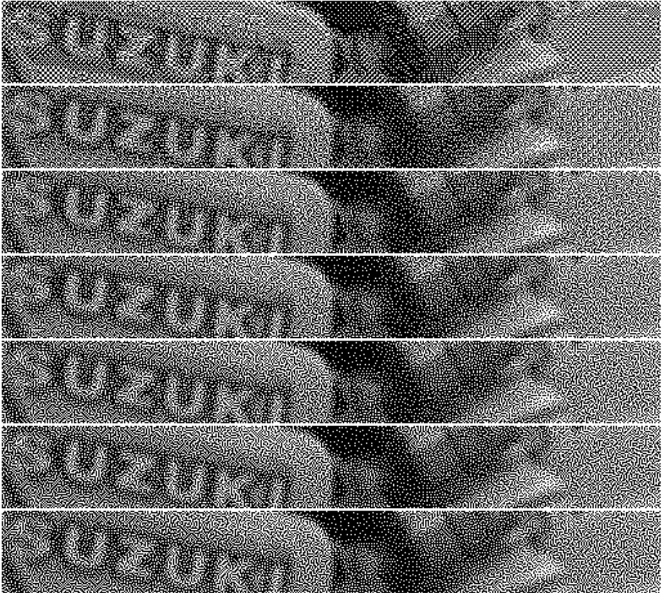
Figure 8. Comparison of image quality for various block sizes from 2 \times 2 (top), 4 \times 4 , 6 \times 6 , 8 \times 8 , 10 \times 10 , 12 \times 12 , to 14 \times 14 (bottom) for the photo part of the image.
