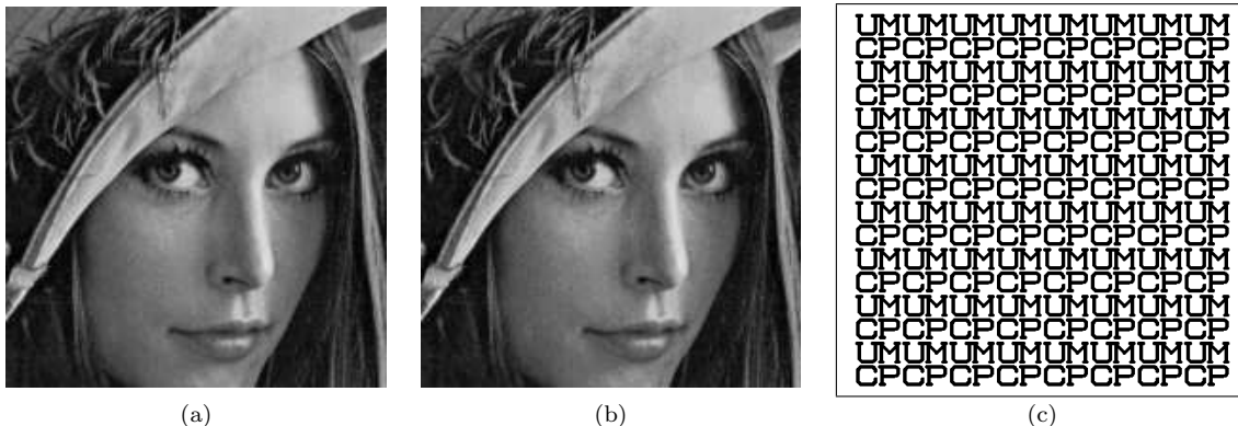
Figure 8. A zoomed-in view of the original Lenna image (a) and the watermarked version (b) using distortion compensated LUT embedding with run constraint of 2, along with a 512 \times 512 -bit pattern (c) embedded in the Lenna image.
