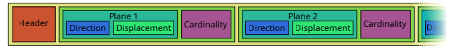
Figure 11: Output bitstream. The header describes the root cell and total cardinality. Each section provides three elements: the bisecting plane direction and its displacement, and the cardinality.
