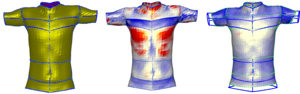
Figure 29: Shrink wrapping a T-shirt mesh onto a body in the rest pose. Left: shrink wrapped T-shirt mesh obtained by solving a Poisson equation that uses a guide “cage” (in blue) as a boundary condition to morph the T-shirt mesh onto the body. Middle: this initial version has area distortion, where red indicates stretching and blue indicates compression. Right: after simulation, the distortion has been reduced and more uniformly spread out so that the cloth pixels can be embedded at better locations. Note that since the T-shirt is constrained to be on the body surface, distortion is not fully eliminated.
