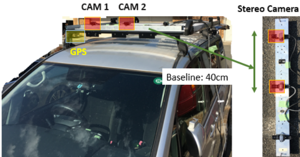
Fig. 5. Experimental setup to collect real traffic data
